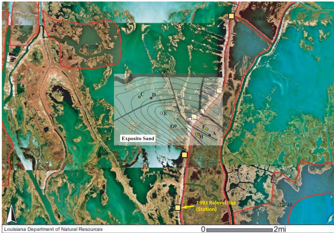
Figure 5.9: Composite diagram (above) showing the structural map for Exposito Sand along with the wells overlaying the aerial photographs. 3 compartments are identified based on the pore pressure history from Figure 5.8 (left). Notice that these compartments seem to correspond with the location of subsurface faults. In other words, the fault might have acted as a barrier within the sand. The structural contour maps are collected from the Department of Natural Resources of Louisiana in Baton Rouge.
