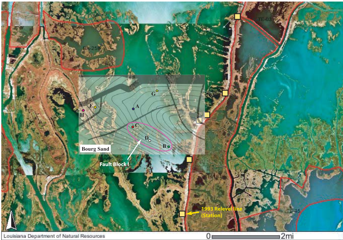
Figure 5.10: Composite diagram for Bourg sand (above). Compartment 1 is identified from the pore pressure history (left). Fault Block IV (or well J in Figure 5.8, left) is located outside of this structural map and will not be considered in this study.
