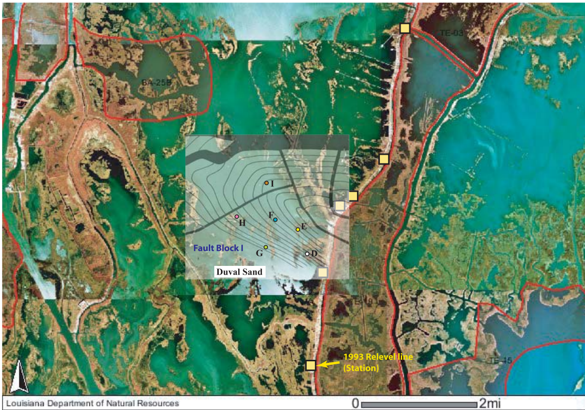
Figure 5.12: Composite diagram for Duval Sand similar to Figure 5.9. Well D, E, F, G and H are drilled within Fault Block I but the pore pressure history suggests the possibility of subcompartments within this block.
