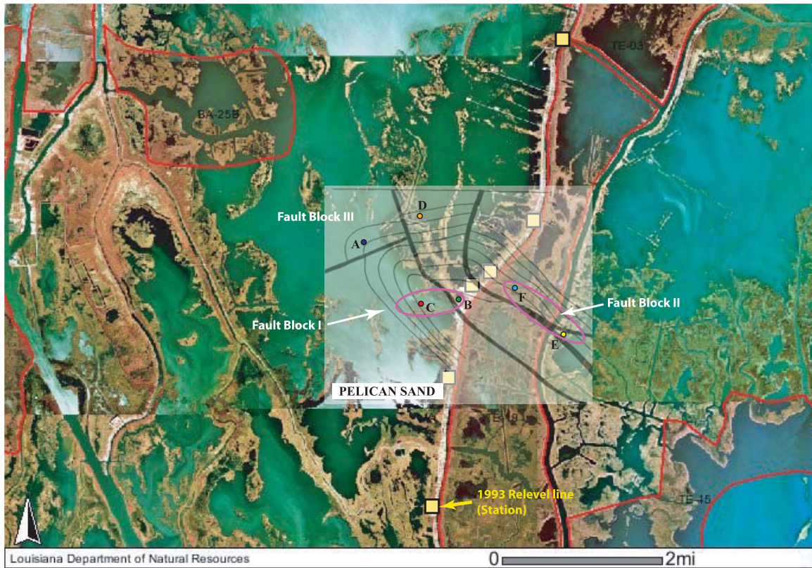
Figure 5.11: Composite diagram (above) showing the structural map for Pelican Sand along with the wells overlaying the aerial photographs. The 3 compartments are identified based on the pore pressure history from Figure 5.8 (left). Fault blocks identified from the pressure history plot and structural map corresponds extremely well suggesting that the faults that separate these compartments are good barrier for lateral fluid movements.
