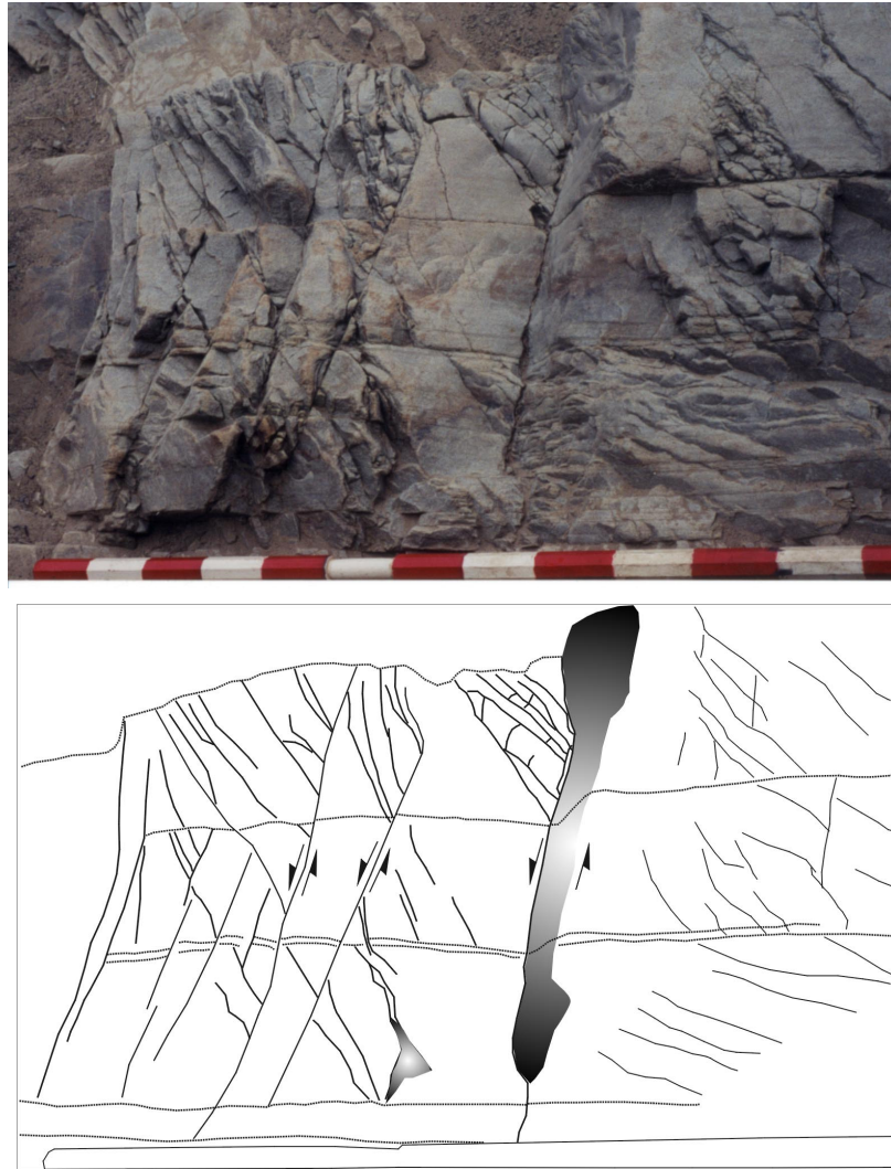
Figure 7.4. Subvertical splay joints, formed due to slip along bedding planes, constitute new weak planes along which shear failure may occur. Slip along these splay joints (arrows indicating shear) generates a new stress perturbation that creates new splay joints. If the failure is dip-slip, as this case, these new splay joints will have the same azimuth as the previous ones but opposite dip direction.
