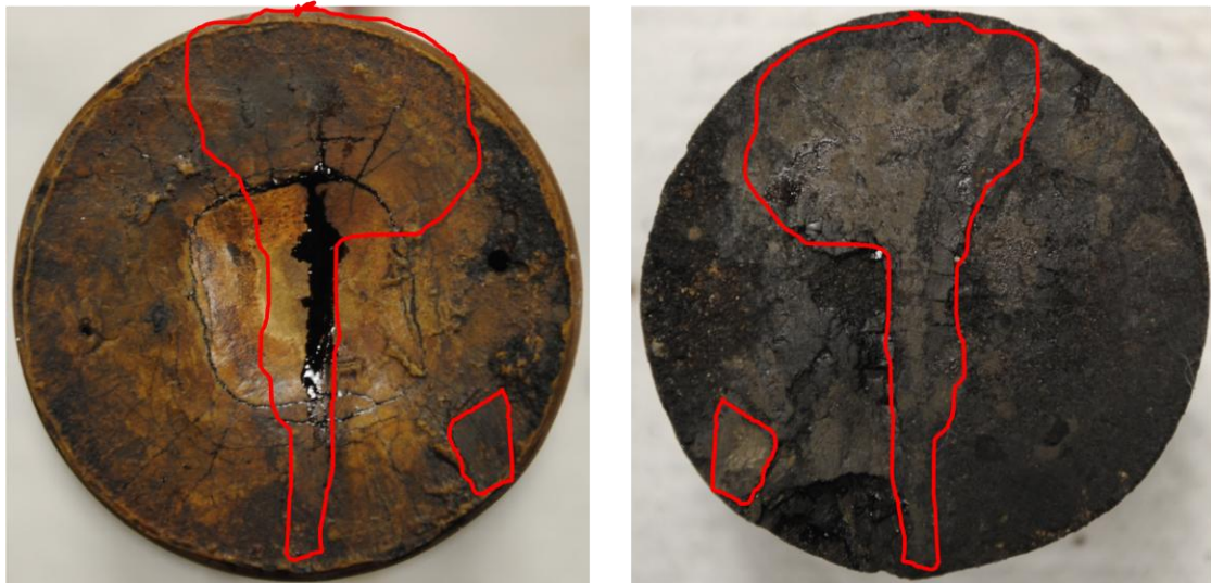
Figure 2.24: Photographs of the Torlon endcap (left) and end of sample S3(right) with pyrite. Note that the pyrite outlined on the sample can be re-aligned with the transducer due to impressions in the Torlon. The main fracture in the end cap aligns with the edge of the pyrite clast.
