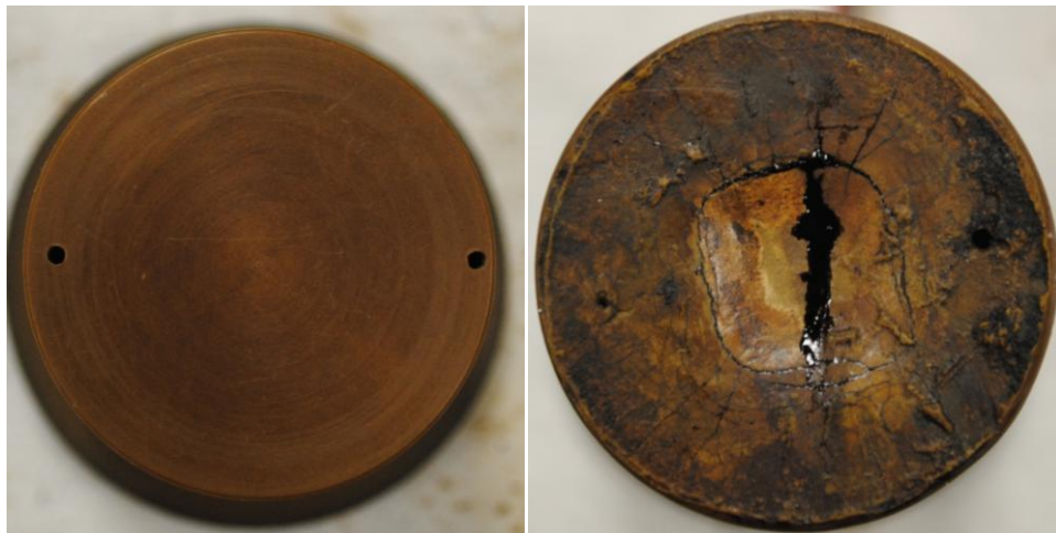
Figure 2.21: Photograph of modified transducer design before (left) and after testing (right). Note that numerous fractures and impressions on the face of the transducer after testing. In particular, there is a pronounced fracture running vertically in the picture that is oozing black bitumen.
