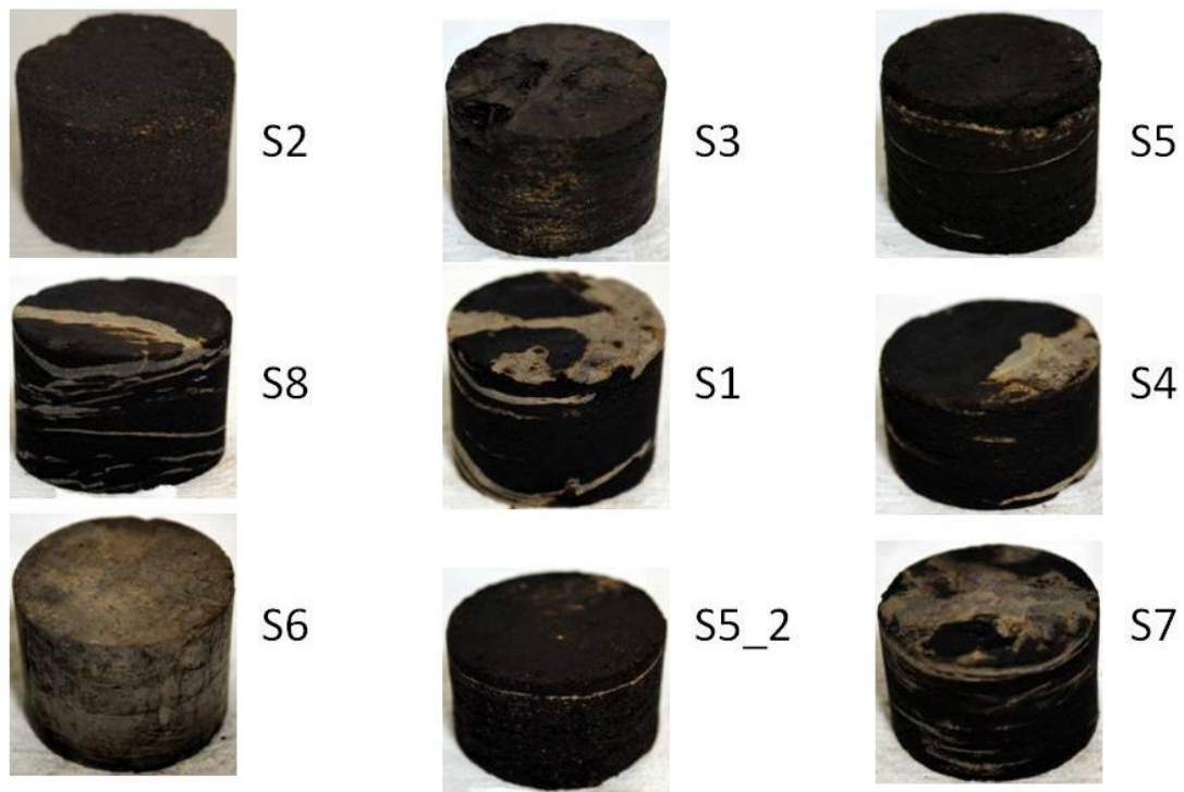
Figure 3.12: Pictures of each of the eight 1.5” diameter samples tested. Note that sample S5 has been cut into two individual samples identified as S5 and S5_2.
