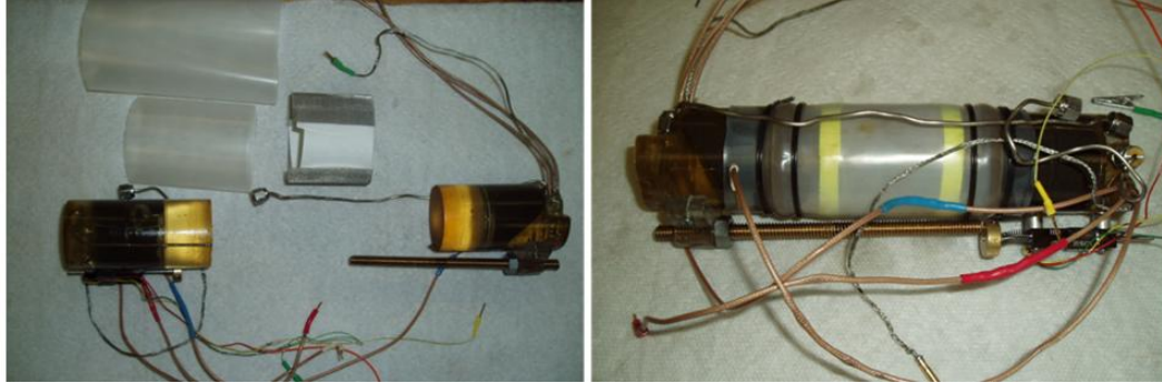
Figure 3.6: Sample preparation for the core sample from a bitumen reservoir. The sample is mounted between two impedance matched transducers, and covered by filter paper, a fine metal screen, and two layers of Teflon shrink wrap.
