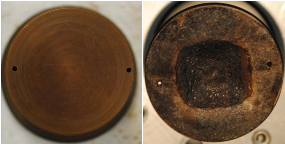
Figure 2.18: Photograph of original transducer design before (left) and after testing (right). Note that the transducer has collapsed into the hollow back where the crystals are mounted.
