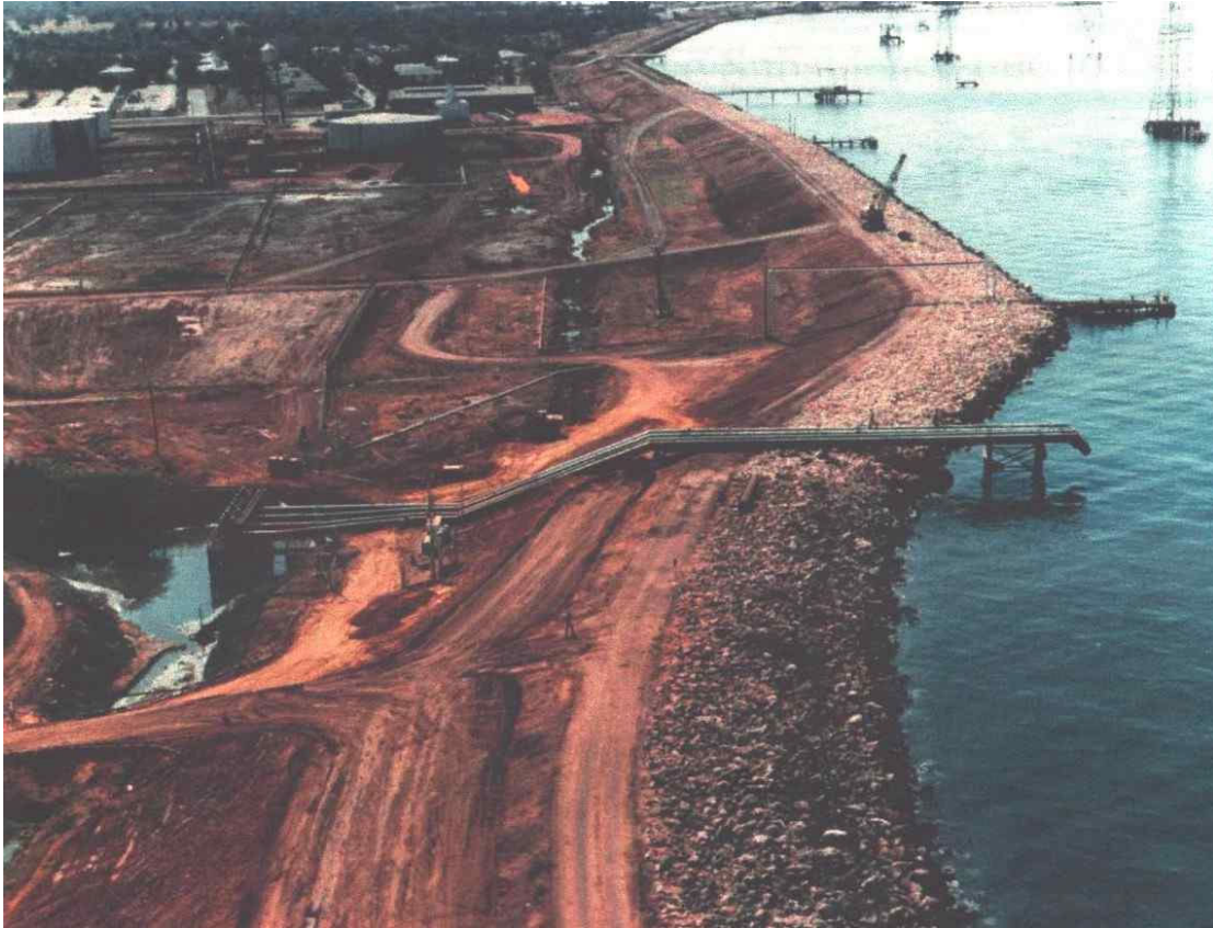
Figure 1.2: Surface subsidence near Lake Maracaibo, Venezuela, due to production of heavy oil (from the Internet).
