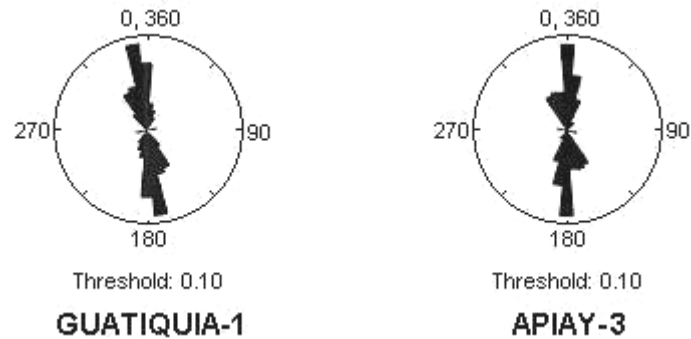
Figure 4.18: A summary of breakout orientation data from the analysis of four-arm caliper logs in two wells of the Apiay-Guatiquía field (adapted from Last et al. , 1997). S_{Hmax} is inferred to be perpendicular to the dominant breakout orientation.
